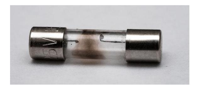
1. This fuse has blown quickly enough so that a metal film deposited on the inside of the glass tube. At high voltages, this film can carry current. (Courtesy of flickr)
