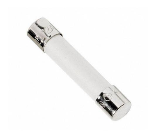
A Littelfuse 1000-V fuse has a ceramic tube. The current, voltage, and speed rating, as well as the safety certifications, are embossed in the metal terminals. (Courtesy of Littelfuse)
